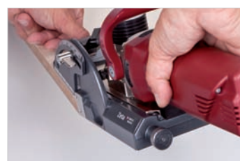
1. Cut the profile groove with the Lamello Zeta
