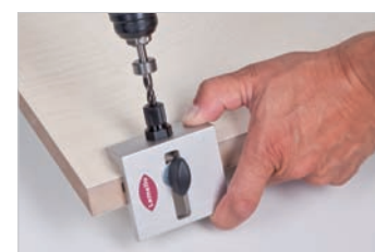
2. Slide the drill jig into the groove and drill the access hole
